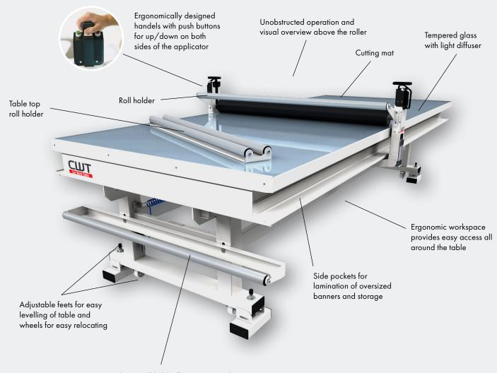
Extra lower roll holder for easy unwinding, storage and feeding of work material
