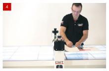
Pull the adhesive material halfway over the roller.
