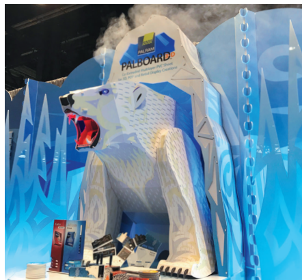
GlobalShop 2019 display fabricated with 5mm and 10mm thick Palboard 3D, white/white/white. No adhesives. No fasteners. All tab and slot construction.
