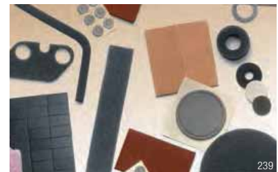
For precise fit, 3M™ Double Coated Tape is pre-applied to foam gasketing materials and then die-cut to size. This helps increase dimensional stability of the part to facilitate assembly.
