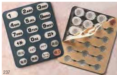
With differential adhesive, the silicone adhesive side of 3M™ Double Coated Tape adheres to a silicone rubber keypad. Acrylic adhesive side adheres to a plastic base.
