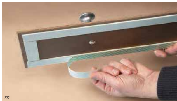
To permanently mount to a textured wall, 3M™ Extra Thick Multipurpose Mounting Tape 4008 bonds on contact and fills gaps between the surfaces.
