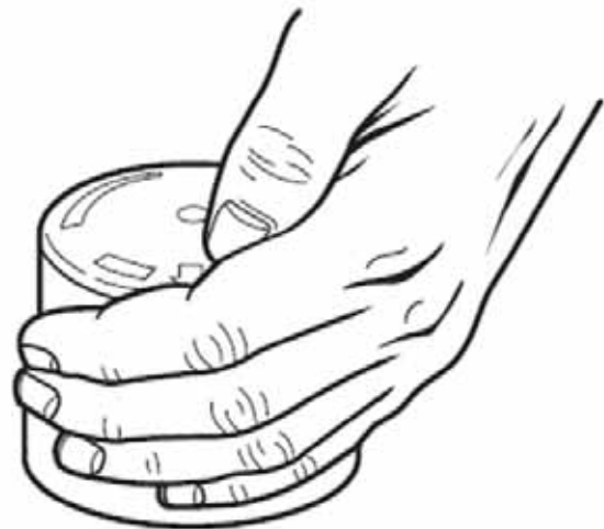
Figure13. Testing photocontrol operation. By gradually exposing the cell to light by moving your hand, you can trick the relay into closing.
