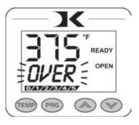
If the OverTemp alarm sounds, set the temperature to a higher value than the current actual temp. Wait 30 seconds and then reset the press to your desired temperature and Watch Carefully. Do not let the press rise to extremely high temps.
