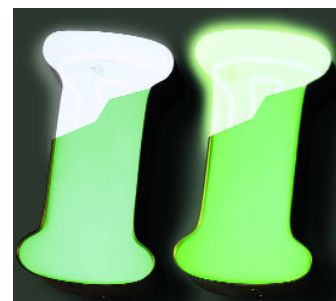
Identical green plastic fascias illuminated by EGL's rare-earth Tropic Green neon tubing (right) are significantly brighter and more vivid than fascias illuminated by conventional white tubing (left).
