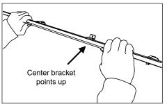
Install ColorLINE sections into clips: Snap ColorLINE sections into mounting clips. Use #6 or #8 pan head screws to secure center bracket once all sections are located on mounting surface.
