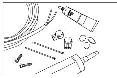
Supplies required: PLTC cable, weather proof 3M<sup>™</sup> Scotchlok<sup>™</sup> UR2 IDC connectors, cable ties, #6 or #8 pan head screws with suitable threads for mounting surface, silicone (outdoor rated caulk), IPS Weld-On #16, and field cut end caps.
