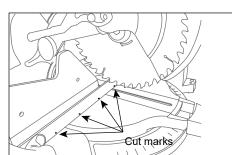
Cutting custom lengths: ColorLINE may be cut on any of black marks (2.4" [61 mm] apart). Use a miter saw to make a clean, straight cut. NOTE: Perpendicular cuts ONLY. Set miter saw to 0°. No angled cuts.
