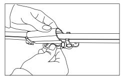
10. **Snap covers into place:** Tuck all loose wires at joints behind ColorLINE extrusion and cover with a joint cover.
