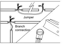
Creating jumpers or branch connections: If jumper or branch connection is required, cut wire or PLTC cable to desired length and use third port on IDC connector as necessary to make connections.
