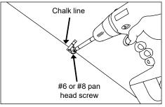
4. Install mounting clips: Snap a chalk line on surface for mounting. Space mounting clips every 12" (305 mm) along chalk line and 1.5" (38 mm) from end of each ColorLINE section. Orient clips with screws towards center of each ColorLINE section.
