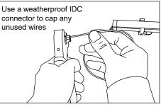
11. Connect ColorLINE chain to power supply: Connect wires from first section of ColorLINE chain to power supply wires using provided Insulation Displacement Connectors (IDC). Connections must be RED-TO-RED and BLACK-TO-BLACK. CAUTION: All primary power supply connections must be made by a licensed electrician. ATTENTION: Toutes les connexions d'alimentation principale doivent être effectuées par un électricien agréé.
