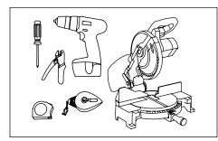
1. **Tools required:** Measuring tape, wire cutters, drill, screwdriver, chalk line, miter saw (for custom cut lengths), and 3M IDC Crimp Tool (part number E-9J).
